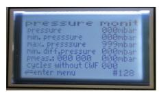
When the control unit switches on the aerator, the pressure within the system should set within a range predetermined by the manufacturer. If the pressure is too low the blower or aerator may be defective or there may be a leak in the hose and pipe system. If the pressure is too high, a valve is
