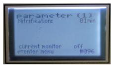
In this menu, the parameter of nitrification and denitrification processes can be modified (optional).
