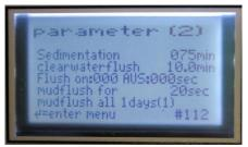
In this menu the parameter for filling, sedimentation and clear water flush can be modified.
