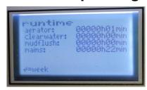
The menu item "runtime" displays the operating hours of the respective aggregate. Hours are added after the Control has switched on the aeration with the corresponding valve. The operating hours of the blower are the sum of the individual running times. The display shows hours and minutes.
